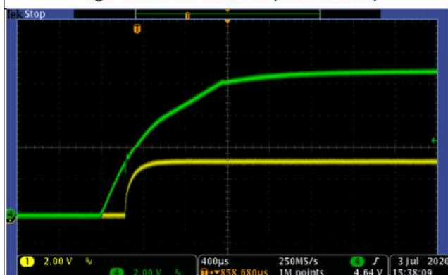
Fig 7 Vout Load Transient (50 to 250mA)
